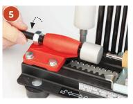
Adjust the end support if needed to push or to support the pen
