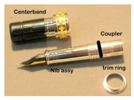
ASSEMBLY: Dissassemble the Centerband assy. (shown in top picture). Now unscrew the coupler from the nib assy. (As shown in bottom picture) Put the trim ring on the coupler with the flat side facing your pen blank, press the coupler into the brass tube.
