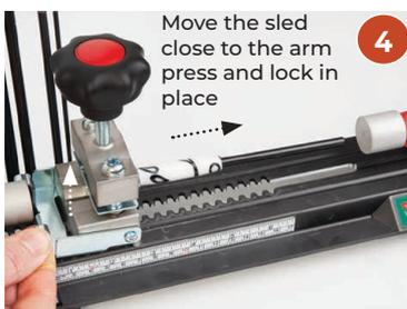
Move the sled close to the arm press and lock in place
