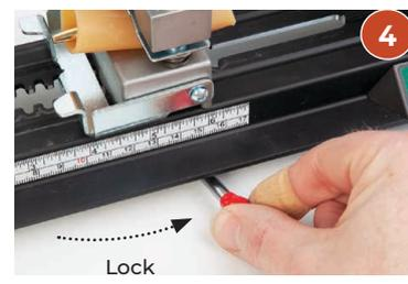
Move the sled closer to the arm press and lock the sled using the clamping lever
