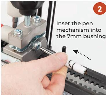
Inset the pen mechanism into the 7mm bushing
