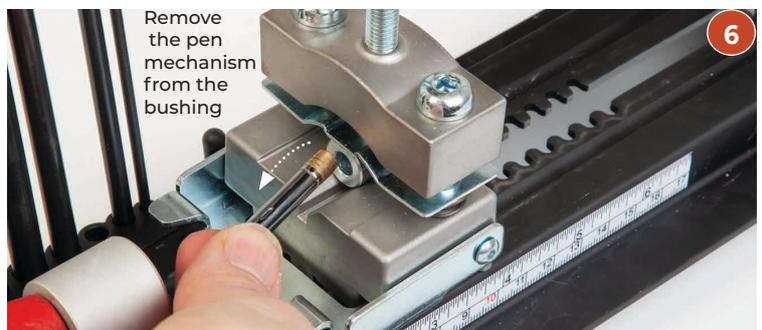
Remove the pen mechanism from the bushing
