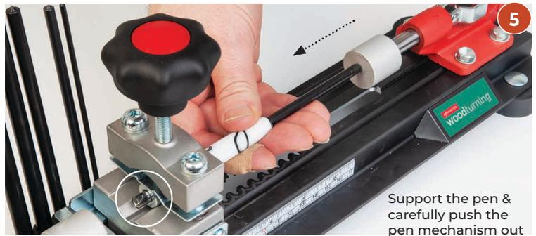
Support the pen & carefully push the pen mechanism out
