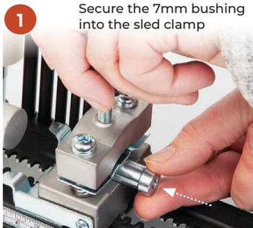
Secure the 7mm bushing into the sled clamp
