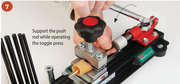
Support the push rod while operating the toggle press
